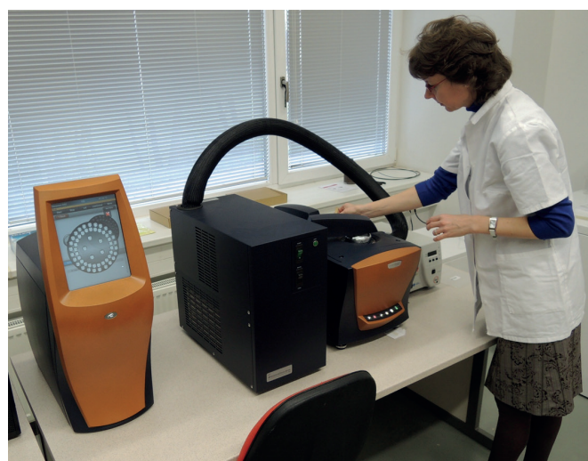
Modulated DSC including Photocalorimeter and endothermic curves of the first and second heating of PA12 with \alpha and \gamma structure
